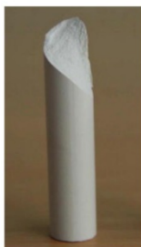
Chalk breakage under torsion
